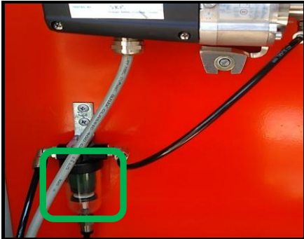
Filter for QT 156 recommend replace instead of cleaning
